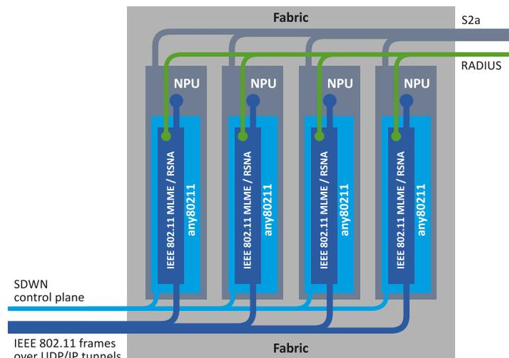
Internal architecture of a Wi-Fi gateway with IEEE 802.11 over UDP/IP tunnel termination software: Incoming IEEE 802.11 over UDP/IP tunnels are split up onto separate NPUs by a hardware load balancer and terminated in the link library (“any80211”). The resulting Ethernet frames are handed over to the surrounding process (TWAG) for further eastbound processing.
