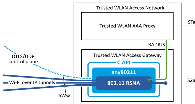
*The Gateway Software and its place in a 3GPP Trusted WLAN Access Network: Authenticating WLAN UE using RADIUS towards the Trusted WLAN AAA Proxy (TWAP) and delivering Ethernet frames between WLAN UE and the Trusted WLAN Access Gateway (TWAG). RADIUS is used for AAA and change of authorization (CoA). All communication with the outside world goes through a C API.*
